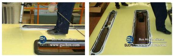
4. Put the shock pad on the pre-processing bolt's or installation hole's location, and glue the bottom of bolt or shock pad before put on them.
