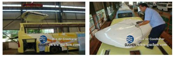
2. Sticking the sponge all around the air outlet and air return on the roof of the bus, please ensure there is airtight and no space.
