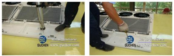
8. Install the bolt into the stuck installation hole, or tight the nut, spring pad, washer, then glue them.
