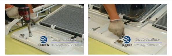
9. Connect the condenser and evaporator, daub the refrigeration oil or frozen on the O-ring when connecting.
